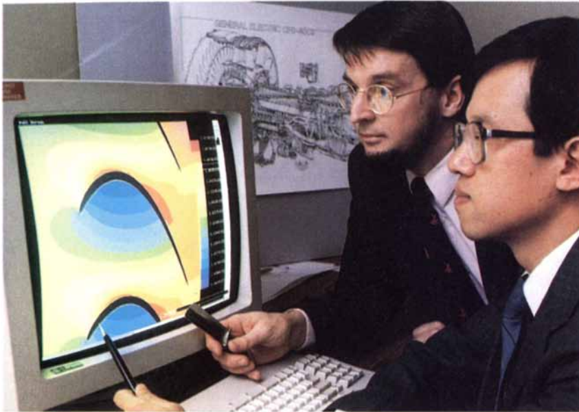
SOFTWARE TO DESIGN JET TURBINE includes a genetic algorithm that combines the best features of designs produced by other programs. Engineers using the algorithm achieved better results than with more conventional software aids.
