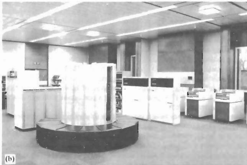
Fig. 1.1 Two modern computers. (a) The PERQ computer, marketed in the UK by ICL: a single-user graphics workstation capable of fast numerical calculations. (b) The CRAY 1-S computer: a supercomputer which uses pipeline processing to perform outstandingly fast numerical calculations.
